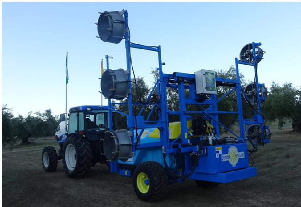
Figure V-9. P2 prototype with six individual axial fans.
