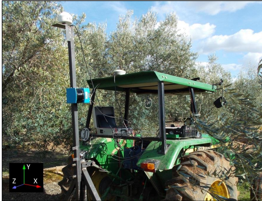
Figure III-5. LiDAR sensor and laptop computer in the field, installed on the tractor.
