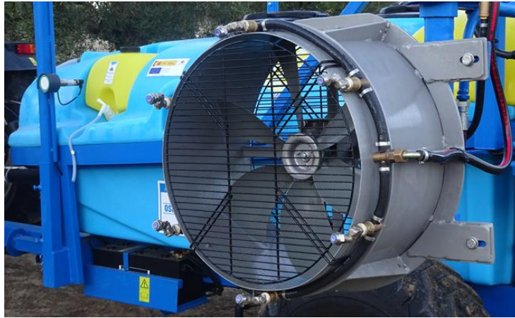
Figure V-11. Axial fan with nozzles and commanding ultrasonic sensor on the prototype P2.
