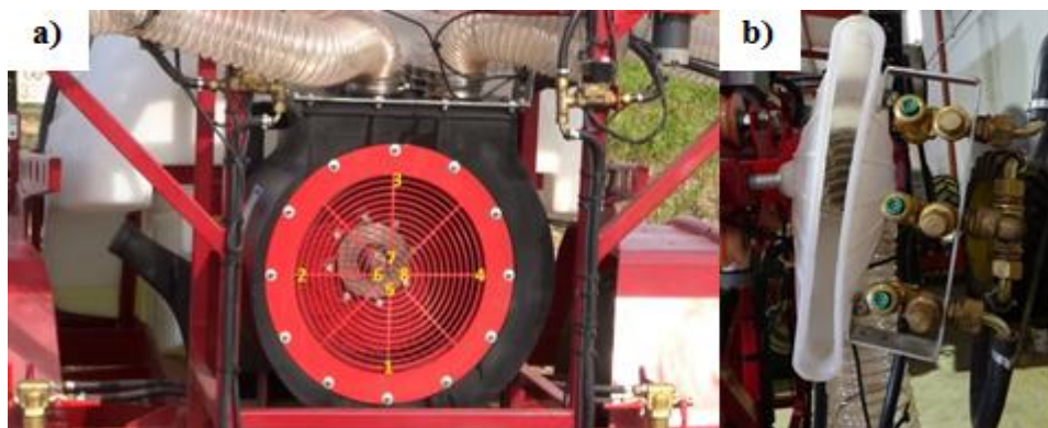
Figure V-7. Components of prototype P1. a) Centrifugal fan. b) Air outlets and nozzles.
