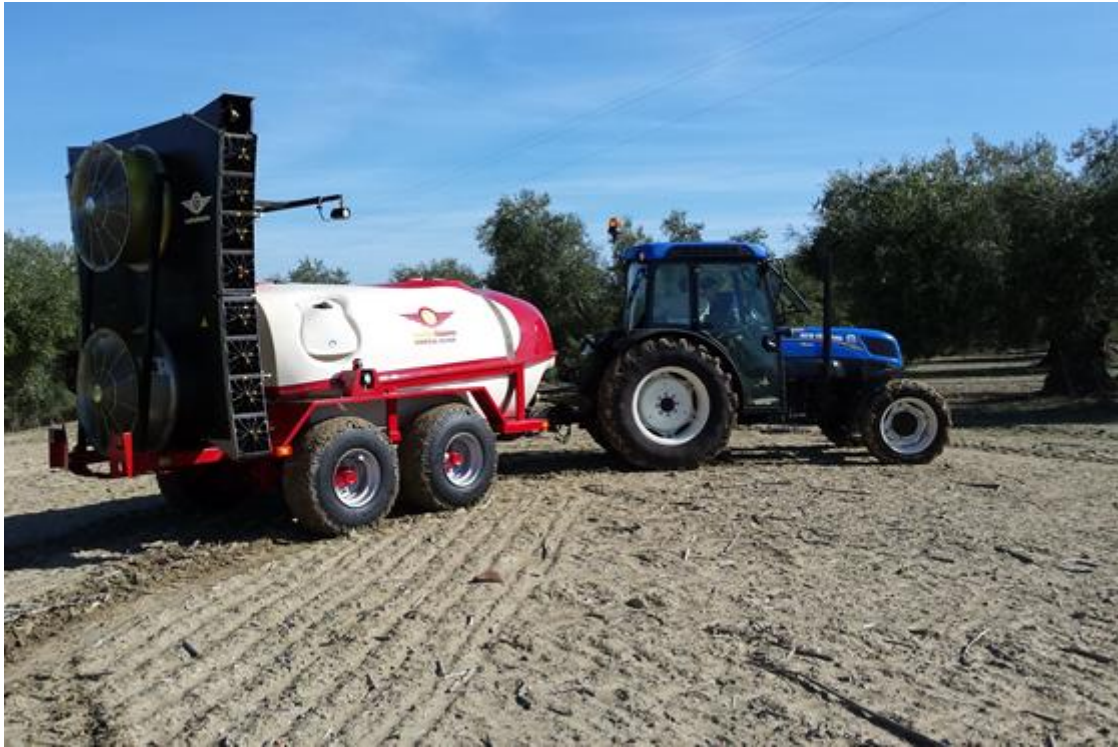
Figure V-12. P3 prototype with two axial fans.
