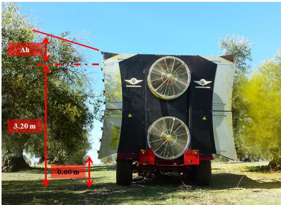
Figure V-13. Application unit position and height in P3.
