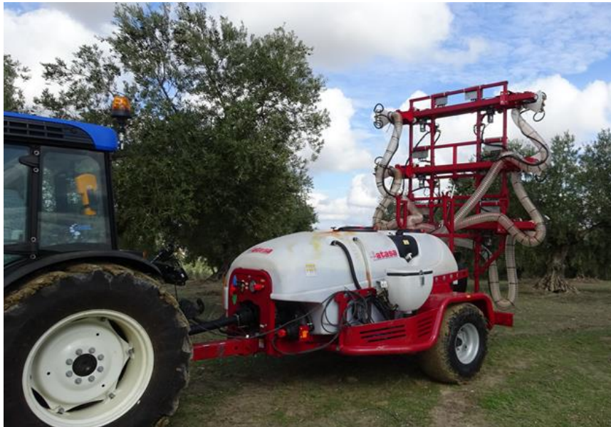
Figure V-5. P1 prototype with central centrifugal fan and individual air outputs.
