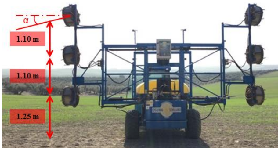
Figure V-10. Heights of the P2 application units and regulation of the top fans to adapt to different tree heights.
