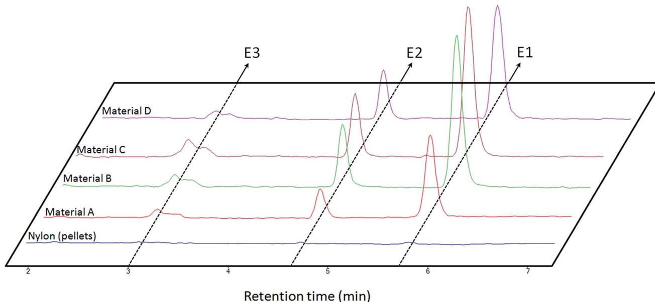
Fig. 6 Obtained chromatograms for the extraction of 1 mL of aqueous standards containing the analytes [estrone (E1),  $\beta$ -estradiol (E2) and estriol (E3)] at the same concentration ( $1 \text{ mg L}^{-1}$ ) by different materials (see Table 1).
