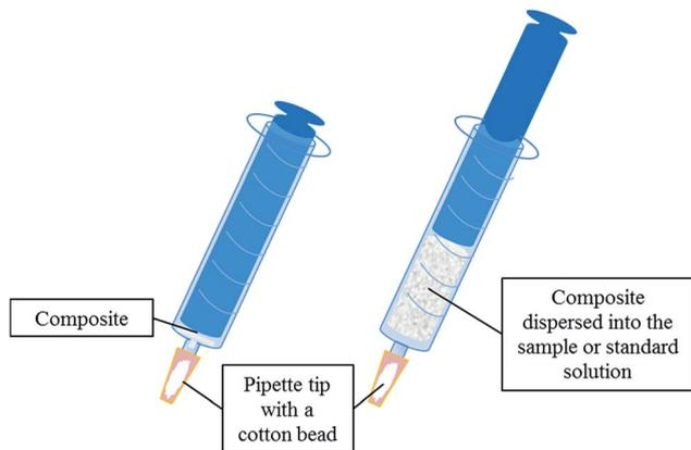
Fig. 1 Schematic diagram of the extraction device used in this work.
