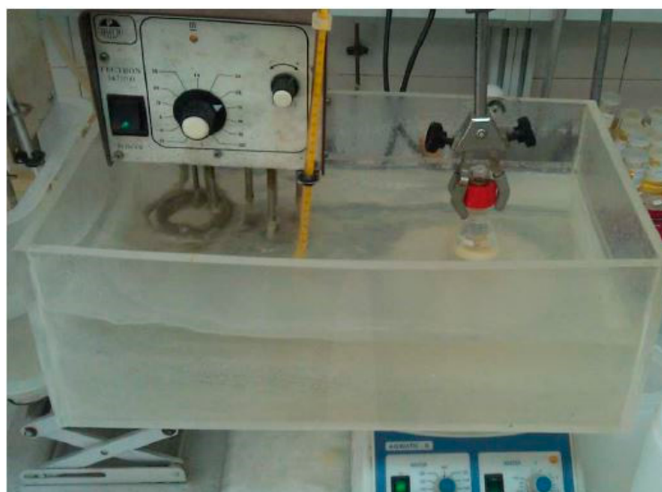
Figure 11. Experimental dispositive for the transesterification reaction.
