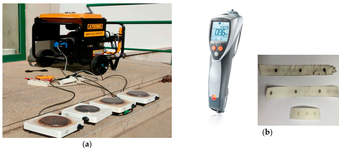
Figure 12. (a) Electrogenerator AYERBE, 5KVA, 230v tipo AY4000MN, heating plates of 1000 watts of power each and voltmeter-ammeter devise (yellow colour, on the floor); (b) TESTO 308 opacity meter, which operates as established by ASTM D 2156-94, Standard Test Method for Smoke Density in Flue Gases from Burning Distillate Fuels.
