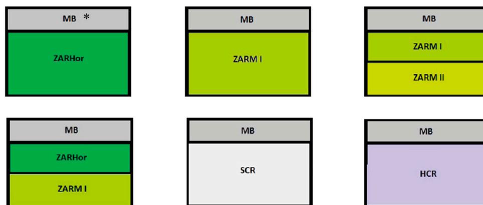
**Figure 1.** Types of structural sections recommended in the catalogue. \* MB = Bituminous mixture.
