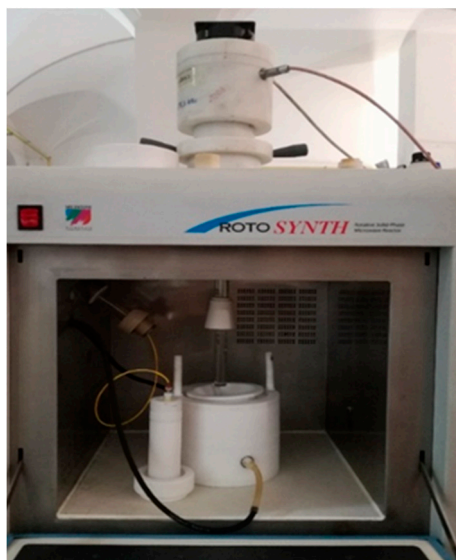
Figure 8. Combined MW/US device.
