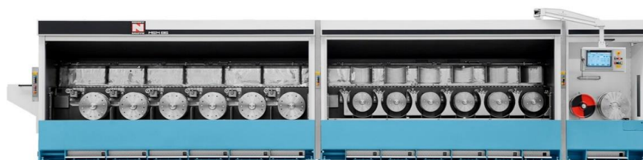
Figure 1. The Niehoff MSM-86 multi-stage wiredrawing industrial machine (Niehoff Stranding Technology, Badalona, Spain) with a maximum of 12 stages used to produce the final wire.
