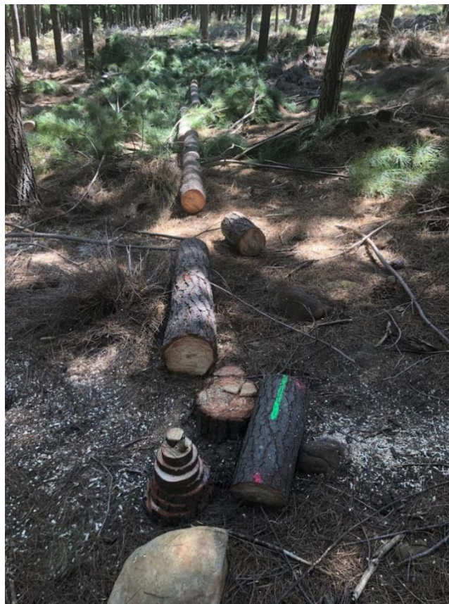
Figure A.3.2. Discs and billet obtained from a tree
