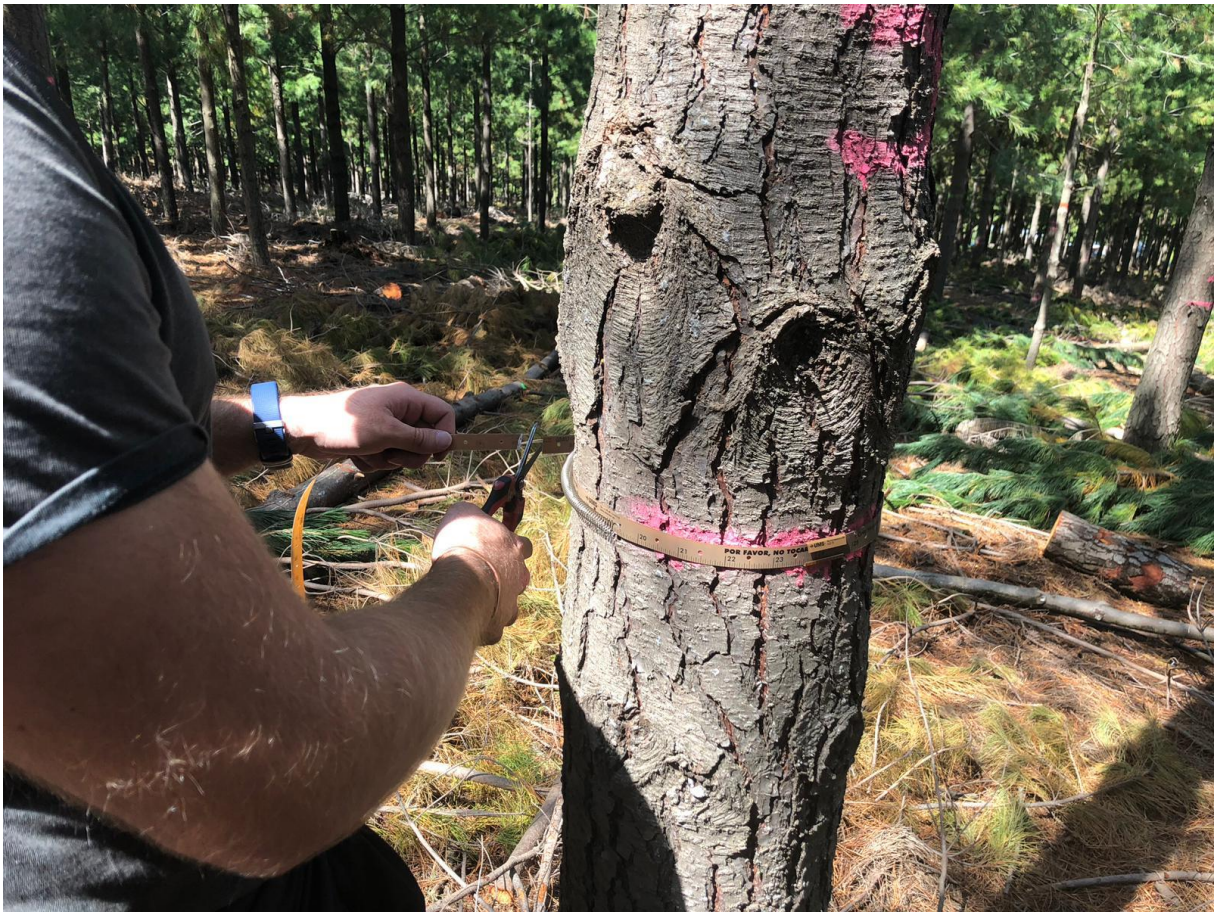
Figure A.3.9. A new installed dendrometer on one of more than 100 trees
