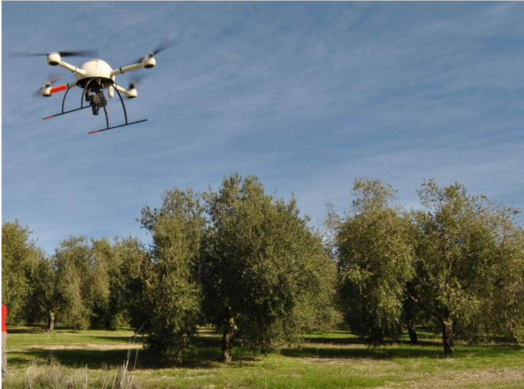
Figure 10. The quadcopter UAV and the Red-Green-Blue (RGB) camera used to acquire the remote images of the olive trees.
