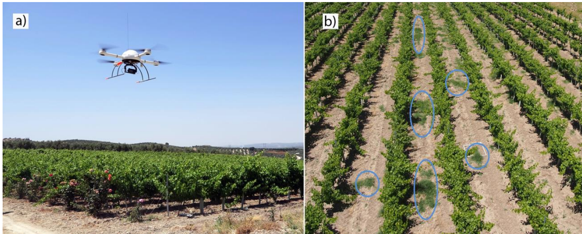
Figure 1. a) Quadcopter microdrone MD4-1000 with the Red-Green-Near Infrared (RGNIR) camera attached, flying over one of the vineyards and b) detail of an RGB-image taken by the UAV from field A-2017. The circles in blue color represent bermudagrass patches growing in the inter-rows.
