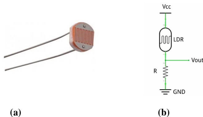
Fig 5. (a) Light dependent resistor (LDR) photo-resistor; (b) Schematic sensor design.
