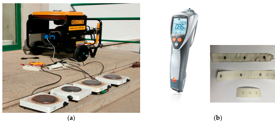
Figure 1. Electrogenerator AYERBE, 5KVA, 230v tipo AY4000MN, heating plates of 1000 watts of power each and voltmeter-ammeter devise (yellow color, on the floor) (a); TESTO 308 opacity meter, which operates as established by the ASTM D 2156-94, Standard Test Method for Smoke Density in Flue Gases from Burning Distillate Fuels (b).
