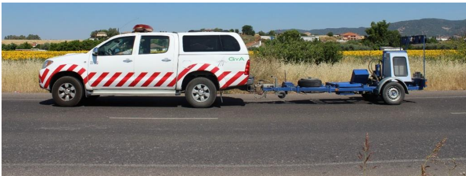
a). Dynatest FWD 8012 – Testing Deflections on ER on 2017
