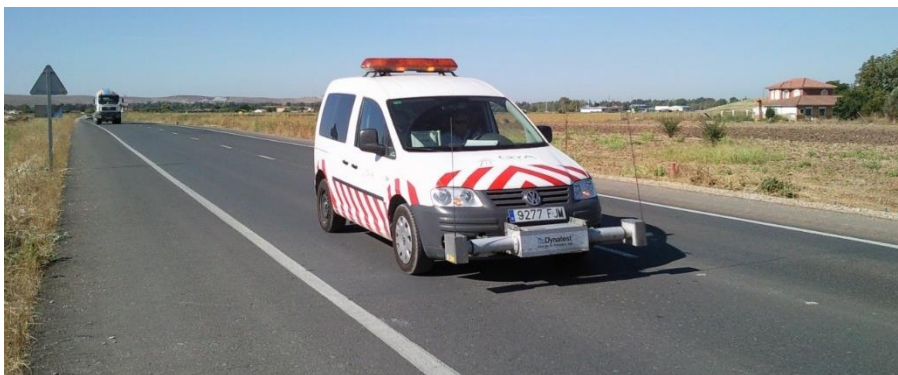
b). RSP MARK-IV equipment – Testing Roughness on ER on 2017
