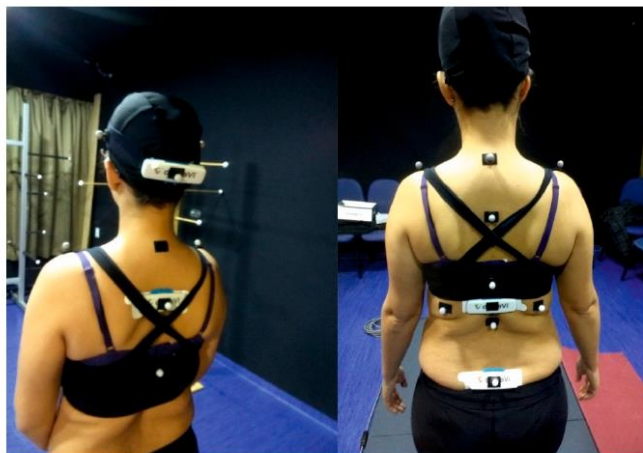
Figure 2. UCOTrack marker set and ViMove sensor location for analyzing cervical and lumbar spinal mobility.
