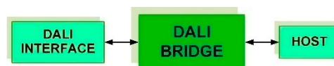
Figure 1. Schematic block diagram of the Digital Addressable Lighting Interface (DALI) Bridge connection.
