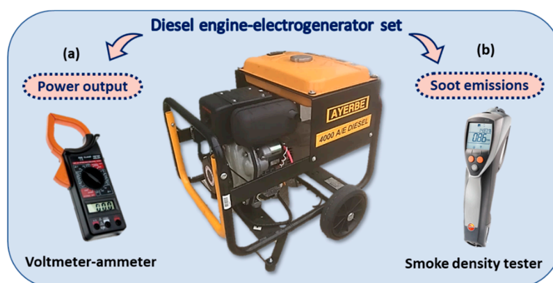
Figure 1. Scheme of methodology on a Diesel Engine-Electrogenerator Set to determine (a) power output by using a voltmeter–ammeter devise; (b) generated soot emissions by using smoke density tester.
