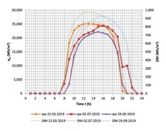
**Figure 6.** Calculated heat flux density per one square meter of an absorber and DNI for selected days for the Solar Thermal Power Station in Spain.
