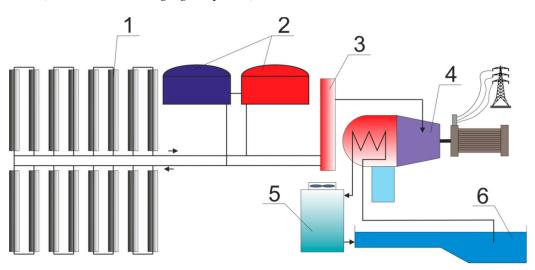
**Figure 2.** Simplified diagram of a thermal power plant with parabolic solar collectors: **1**—parabolic solar collectors, **2**—heat storage tanks, **3**—steam generation system, **4**—steam turbine, **5**—cooling tower, **6**—water storage reservoirs.
