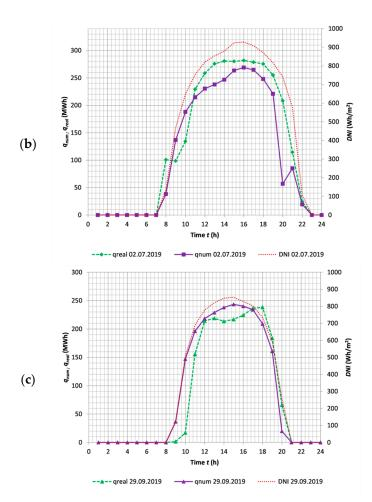
**Figure 7.** Comparison of heat produced by solar collectors with heat determined from the developed model the Solar Thermal Power Station in Spain for selected days: (a) 22.03.2019, (b) 02.07.2019, (c) 29.09.2019.
