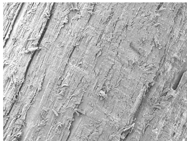
FIGURE 1 Scanning electron microscopy image of the surface of a wooden toothpick at 100x magnifications. Reproduced with permission of Elsevier from reference [52]
