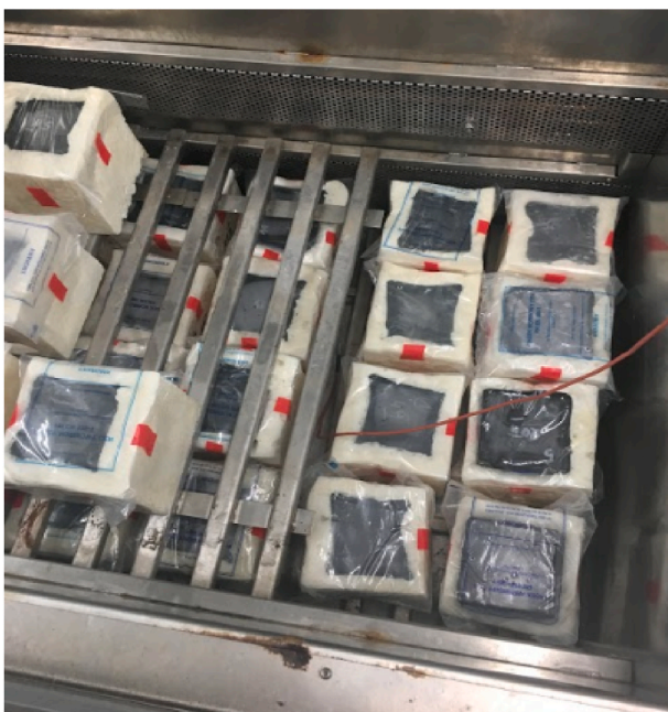
Fig. 1. Geopolymer concrete frost resistance test.
