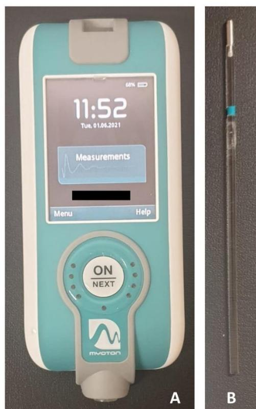
**Figure 2.** MyotonPro<sup>®</sup> device (A) and 100 mm long probe (B).
