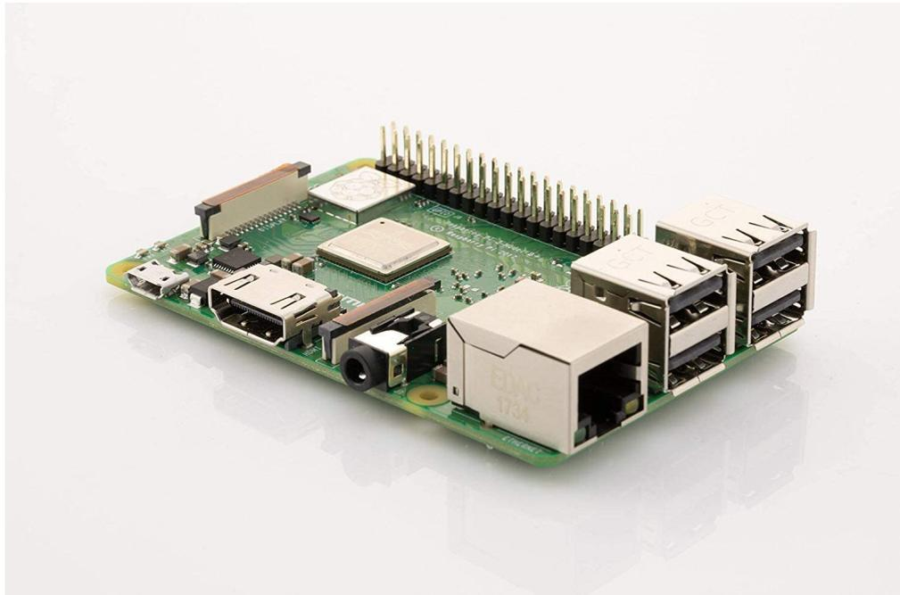
Figura 7 Raspberry Pi 3 B+. Fuente: [www.raspberrypi.org](http://www.raspberrypi.org)
