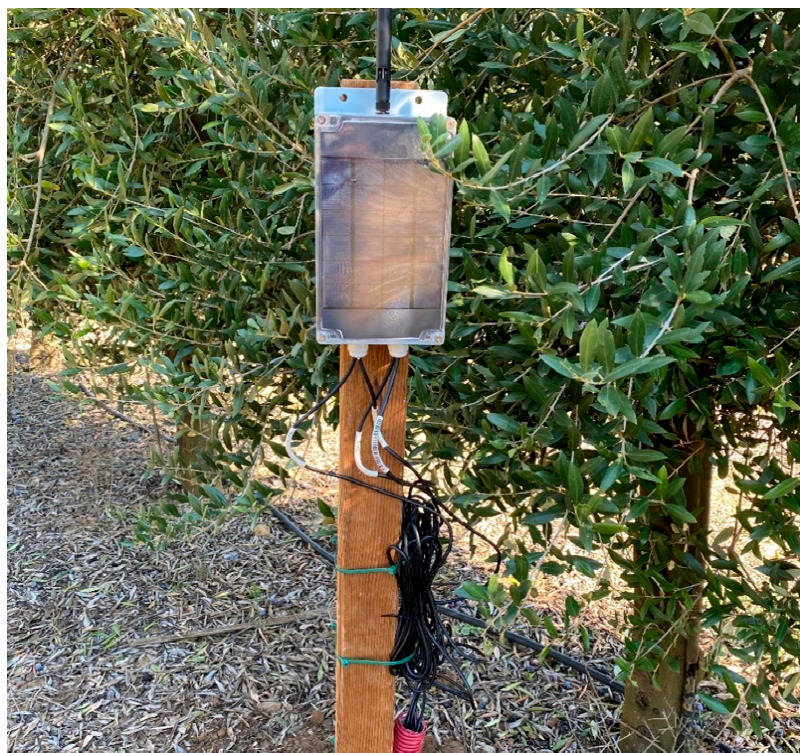
Figure 8. Communication node with connected soil moisture sensors.
