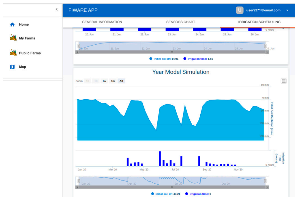
Figure 11. Annual simulation of the irrigation model showing water depletion in the root zone when using the RDI strategy defined in Figure 10 for a high-density olive grove.
