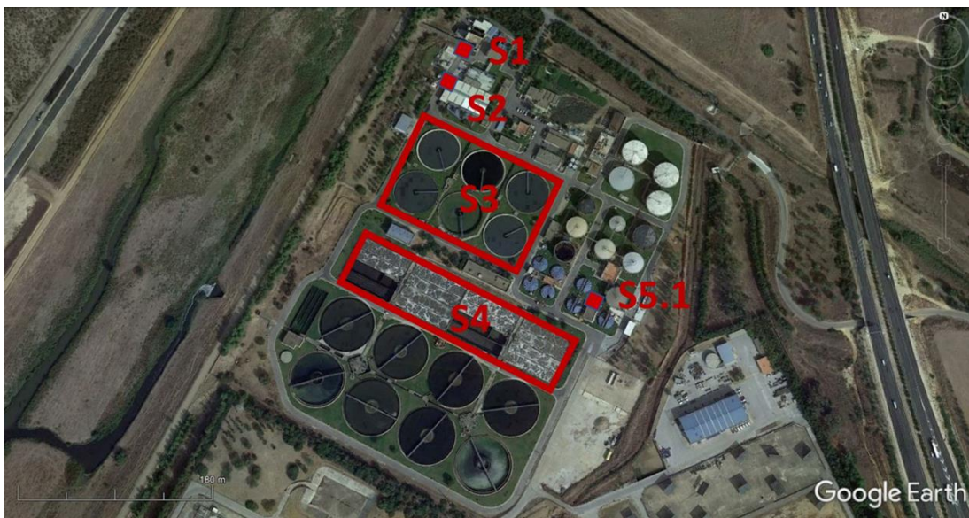
Fig. 2. Outline of the sources considered for the modelling of the odour dispersion (S1, pre-treatment header; S2, sand and fat removal; S3, primary settling; S4, biological treatment; S5.1, gravity thickening).
