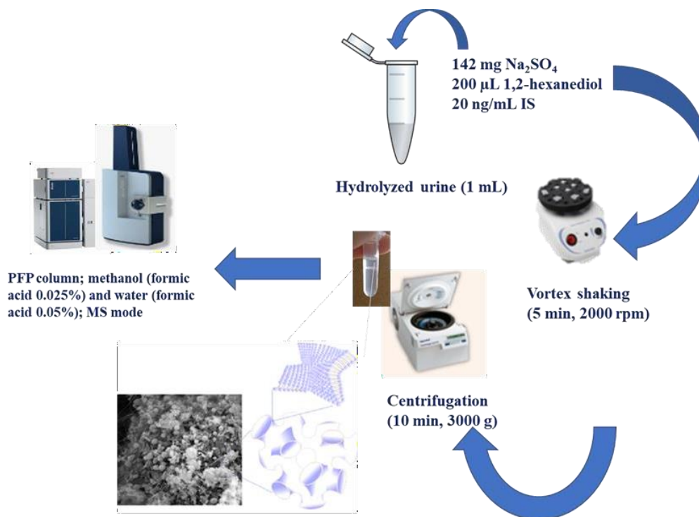
Figure 1. Schematic of the SUPRAS-based sample treatment for screening analysis of multiclass substances in urine by LC-ESI-TOF.
