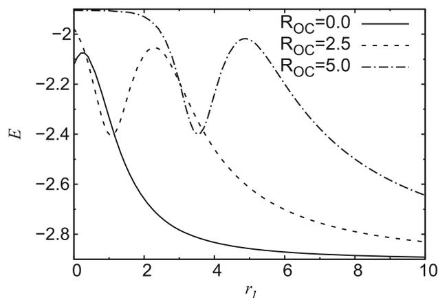
of  $r_1$  which depends on the position of the nucleus inside the MLQD. The energy decreases as the core radius increases, approaching the free atom energy in the case of the on-center configuration.
