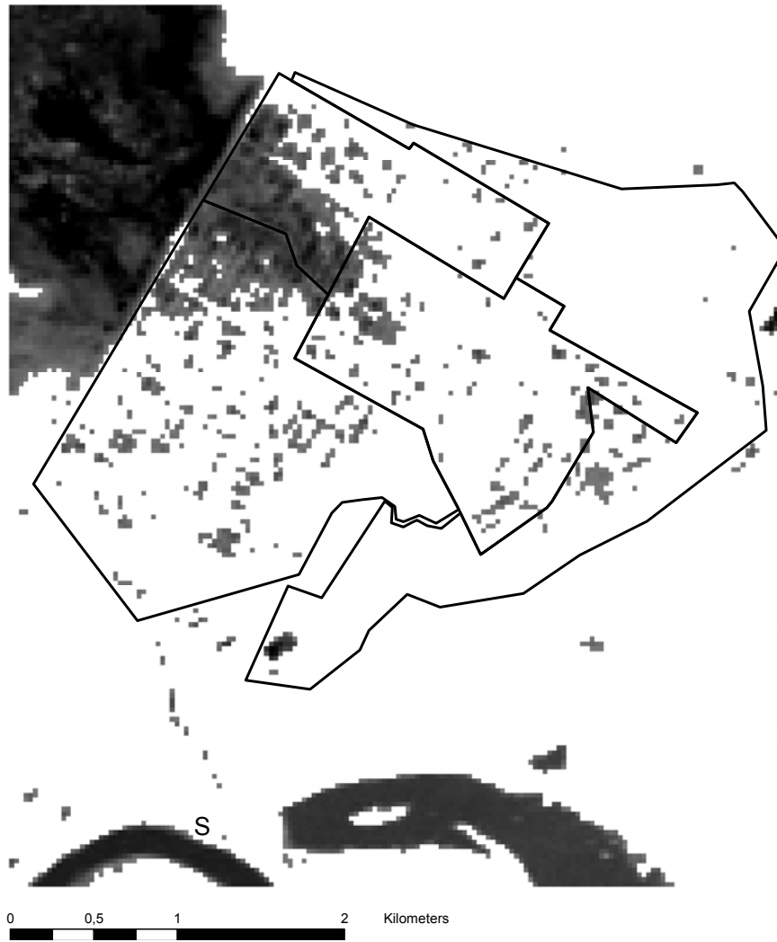
Figure 5.6. Map of drainage problems based on infrared reflectance measured from Landsat satellite over CPB irrigation scheme.
