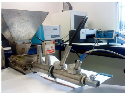
Fig. 1. System designed for this work in order to take Raman measurements.
