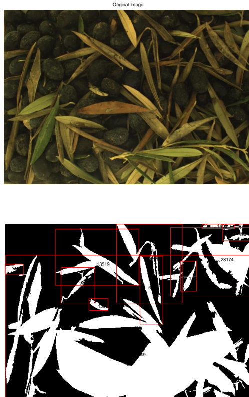
Figure 1. Original image (a) and image after the colour based segmentation, showing the results expressed in the pixel area occupied by leaves (b).
