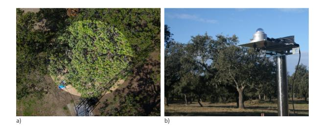
Figure 2.9: a) FOV of the SI111 installed over the oak and b) pyranometer installed in EA1.
