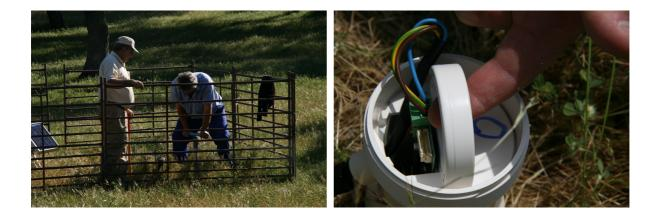
Figure 2.7: Soil humidity probes installed in Santa Clotilde study area.
