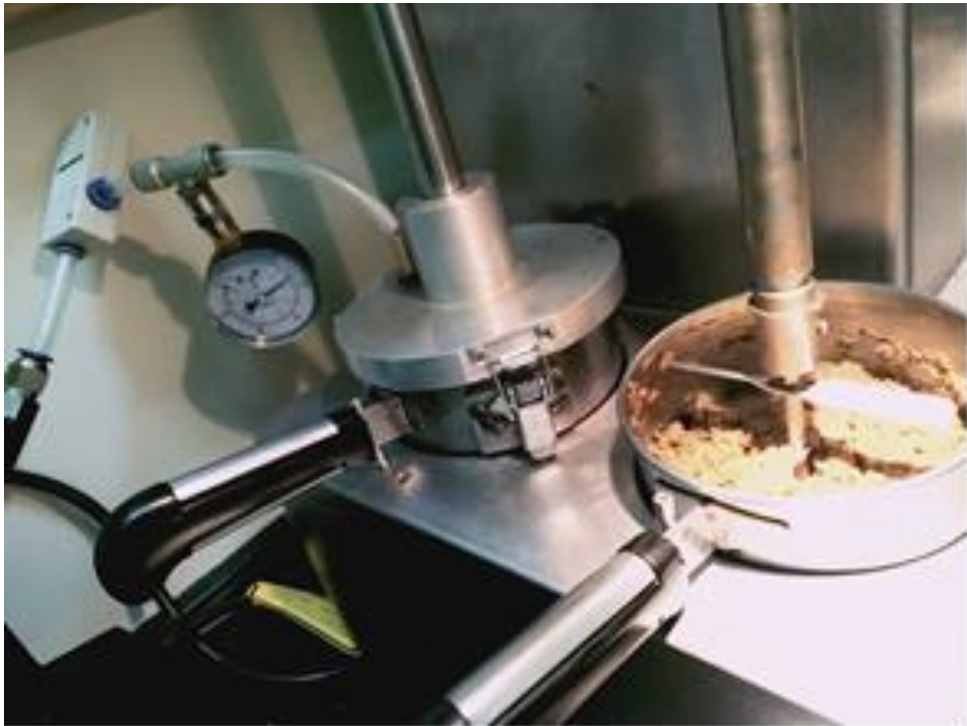
Supplementary figure 1. Experimental set-up installed in the Abencor system to test the effect of vacuum in the malaxation step (left) versus standard conditions (right).
