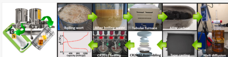
Schematic illustration of the process of manufacturing the cathode of a Li-S cell from brewing waste and battery testing (reprinted from Ref. [266] with permission from John Wiley and Sons).
