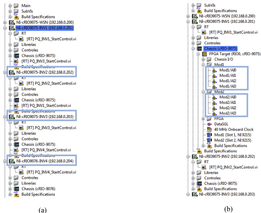
Fig. 6. Configuration of the cRIOs in the LabVIEW project: (a) Detail of cRIOs's configuration; (b) Detail of the acquisition module in a cRIO.
