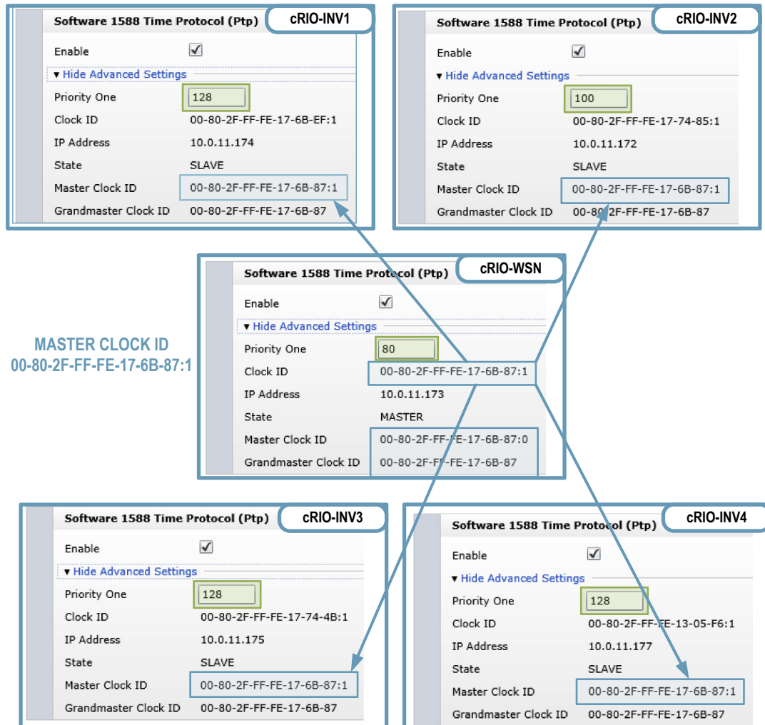
Fig. 15. Configuration of the synchronization system.
