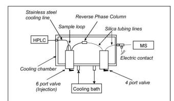
Figure 1. Schematic representation of SAIDE, a semiautomatic interface for DH MS. The scheme shows the components contained inside of a thermostatic box. The temperature probe is located on the sample loop and is set to -2 °C. The system contains the electric contact of the electrospray source. The entire assembly in installed on the front end of a LTQ FT mass spectrometer.
