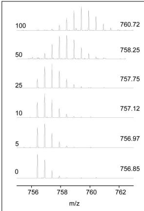
Figure. 3. Isotopic envelopes of a doubly charged peptide-ion reconstituted in different content of D2O. The figure shows the isotopic envelopes for the doubly charged ion of the peptide TDDSQPWVLPVVR dissolved in deuteron-ammonium phosphate containing different amount of D2O. The content in D2O is indicated at the lower left corner of each trace. For each isotopic envelope, its average mass is given on the upper right corner.
