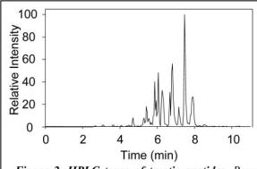
Figure 2. HPLC trace of tryptic peptides. Base peak chromatogram showing the rapid elution of the peptide mixture obtained after trypsin digestion of cAAT. Most peptides elute in less than 10 minutes.
