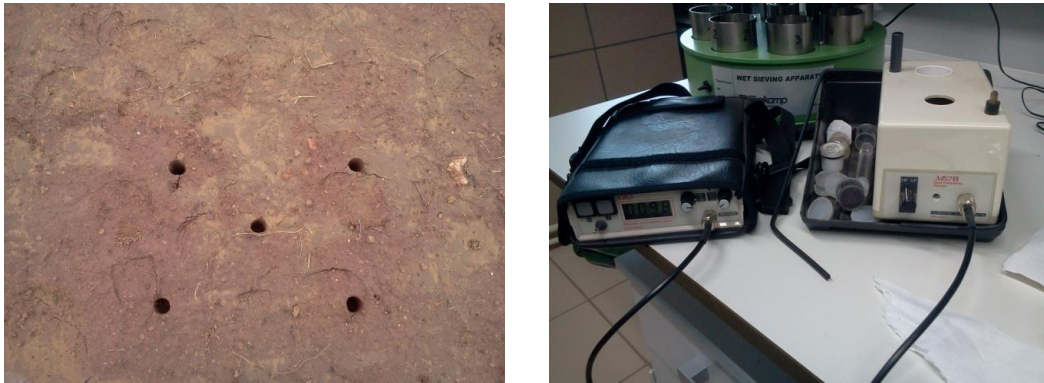
Figure 3.3. Soil sampling for magnetic susceptibility determination (left) and mass magnetic susceptibility in the laboratory (right).
