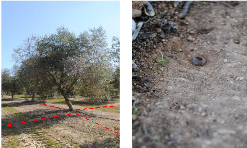
Figure 2.3. Scheme of the sampling transects performed in every olive tree every 10 cm (red lines) and droplet for the assessment of soil water repellency (WDPT).
