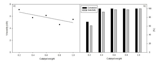
The use of higher catalyst amounts will not promote increasing catalytic activity because under these conditions kinetic control of the reaction does not operate. This indicates that the best experimental conditions are obtained by using 8 wt% of heterogeneous KF catalyst, respect to the amount of oil used.
