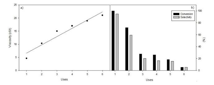
**Figure 7.** (a) Viscosity values obtained in the successive reuses of heterogeneous selective methanolysis of sunflower oil (viscosity 32.0 cSt) under standard conditions, with 0.8 g of KF/ZnO, 65 °C, 12 mL of oil and 2.43 mL methanol. (b) Conversion and Selectivity values obtained with identical conditions.
