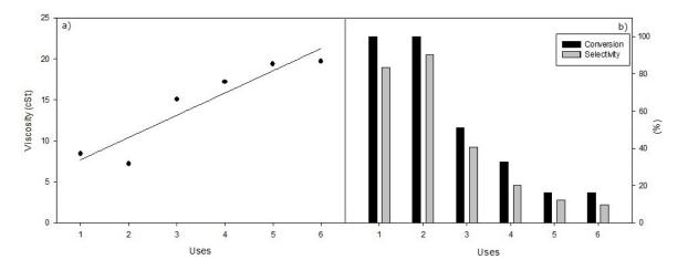
**Figure 8.** (a) Viscosity values obtained in the successive reuses of heterogeneous selective methanolysis of sunflower oil (viscosity 32.0 cSt) under standard conditions, with 0.8 g of KF/MgO, 65 °C, 12 mL of oil and 2.43 mL methanol. (b) Conversion and Selectivity values obtained with identical conditions.
