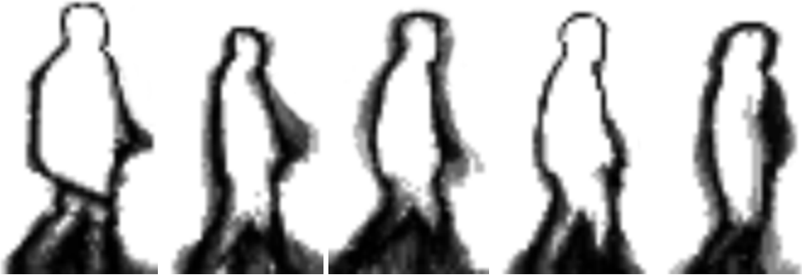
Fig. 2 Several examples of GENI, computed over a gait cycle. The gray level represent the entropy value in a pixel. As can be seen, legs and arms have high gait entropy value, whereas static areas as torso have low values of entropy.
