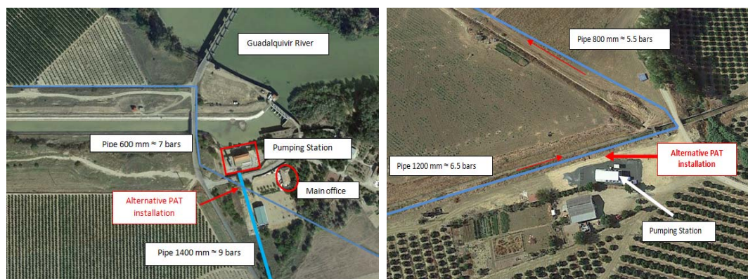
Figure 7. Alternative MHP locations in the irrigation sector.
