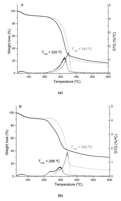
**Figure 4.** TGA and DTG curves for the different cellulose nanofibers: (a) lignocellulose nanofibers (LCNF) and (b) cellulose nanofibers (CNF). Black curves for those obtained by TEMPO-mediated oxidation and grey from mechanical pretreatment.
