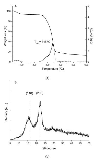
**Figure 1.** (a) Thermogravimetric analysis (TGA) and TGA equivalent derivate (DTG) curves and (b) the XRD pattern of OTBP pulp.
