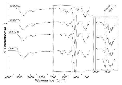
Figure 2. FTIR spectra of the different cellulose nanofibers.
