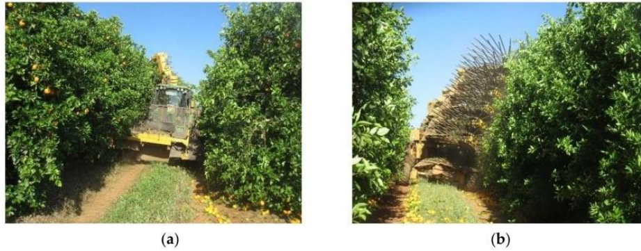
Figure 2. Lateral tractor-drawn continuous canopy shaker system (Oxbo, 3210) used in citrus harvesting tests. (a) front view before the harvesting process; (b) rear view after the harvesting process.
