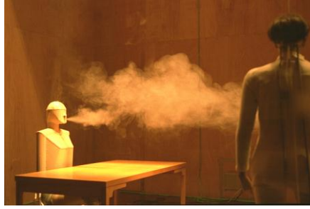
Figure 9. Smoke experiment with two manikins in a room with a vertical temperature gradient. The smoke indicates a layer of high concentration exhaled from the seated source manikin.
