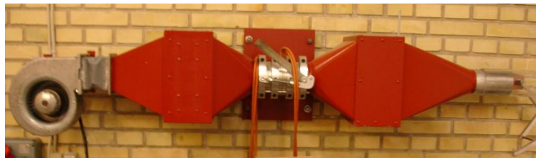
Figure A.4 Wind tunnel where the anemometers were placed to be calibrated
