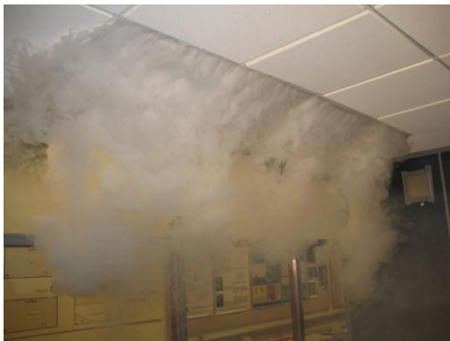
Figure 6 (a) Picture of the airflow generated by the textile diffusers, (b) Sketch of the room with the manikins' positions of test b and placement of the horizontal lines L4 and L5
