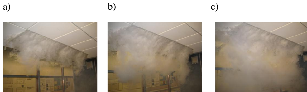
Figure 3.9 Smoke visualization of the flow at three instants of time a) 1s, b) 2.5 s, c) 4.5 s
