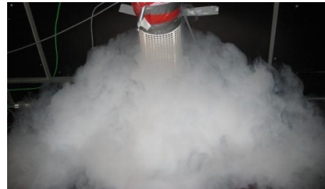
Figure 3.7 a) Velocity profile generated by the wall-mounted displacement diffuser along at horizontal line at 0.01 m from the floor, b) Airflow smoke visualization
